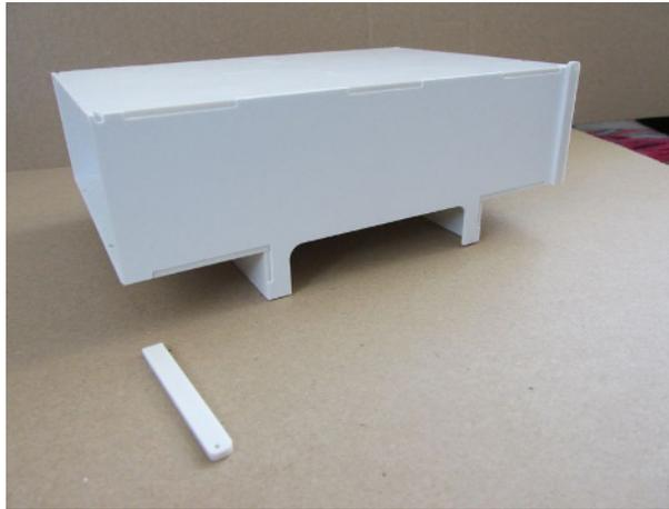
On the box, the bearing strips are adhered now to the four front edges. The hole should come be closer to the forward edge and cover with the slots in the floor.
