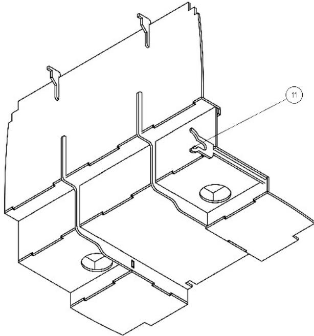
Glue the template (11) for the tilt limiter bearing with only some small glue points a approx. 5 millimeters / 0.19 inch from the edge, after installation of the bearing it can later be removed again.
