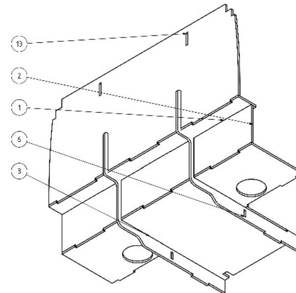
Glue the side parts (6) to the slots in part (3) right-angled and flush fitting and the small dividing wall (2) also right-angled and flush fitting to the floor part (3).
