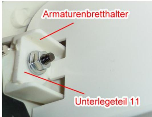
Since the original seat holders are not used, but are missing now as a rest for the collar nut of the dashboard holder, part (11) can be positioned below the collar nut one to the left and one to right. Thus, the dashboard holder is fixed now again.
