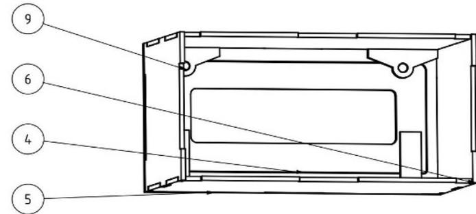
In the two magnet holders (9) each have a magnet (diameter 3 mm - 1 mm thick) is glued so that the magnet surface to the outer side is flush (Magnetic polarity note).
