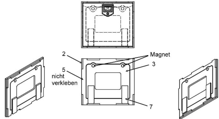
Initially, the lid is assembled, as well as take the frame member (5) as a template to help.
