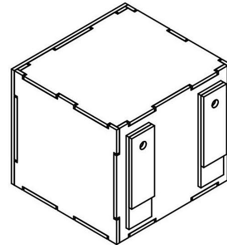
Here in the picture you can see the use of the distance spacers. At its discretion, depending pair a long and short pieces and matching drill holes.
