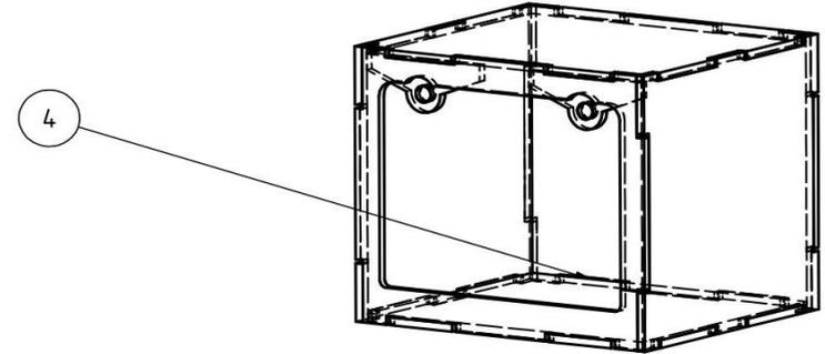
Fit the rear wall (4) back and glue especially all inner edges and the magnetic holder well.
